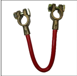
BCCR0300-12 BATTERY CABLE BATTERY TO BATTERY RED / TERM - TERM 16MM X 300MM
